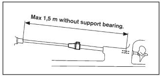
It's crucial that the shaft is within tolerance and straight or the installation may cause damage to the seal and leakage into the boat.
