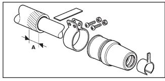
Always make sure that there is a minimum of 36 mm's (A) length at the end of the sleeve to ensure a proper assembly.
