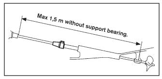
Always install the water lubricated seal under the waterline to ensure proper function.
